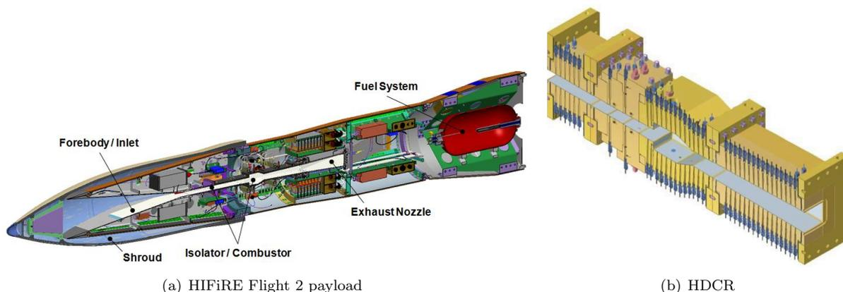
Figure 1. HIFiRE Flight 2 payload and HDCR cut views.
