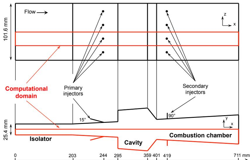
Figure 2. Schematic of the full computational domain.
