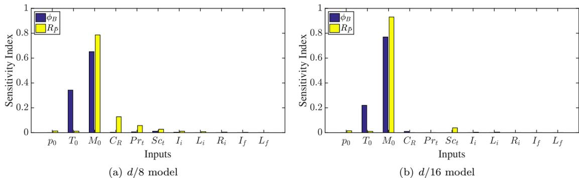
**Figure 3. Sobol indices (total effect sensitivity) for  $d/8$  and  $d/16$  models, QoIs  $\phi_B$  and  $R_P$ .**
